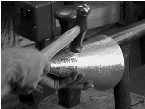
Figure 2: Silver vessel in the process of being formed from flat sheet. Photo: K. Paynter/A. Shillito, 2001
